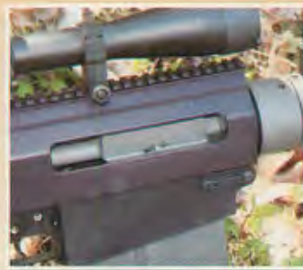
(1) Here the mechanism of the BA-50 can be seen clearly. Note the roller on the bolt. It is one of three. (2) Here the bolt is up, to illustrate the position of the parts just before the bolt is retracted. (3) Here the ejection port is seen in the open position on the right side of the BA-50.
